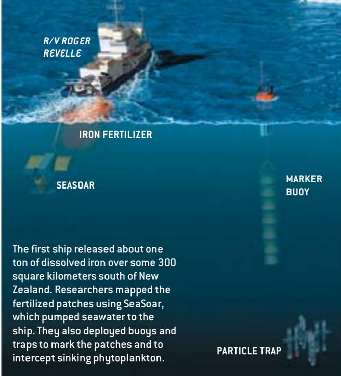
The first ship released about one ton of dissolved iron over some 300 square kilometers south of New Zealand. Researchers mapped the fertilized patches using SeaSoar, which pumped seawater to the ship. They also deployed buoys and traps to mark the patches and to intercept sinking phytoplankton.
